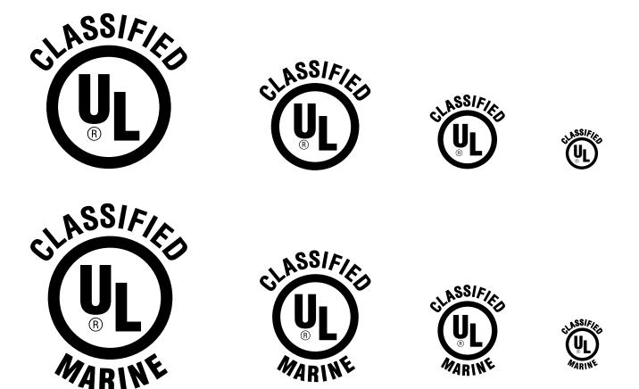
The minimum height of the registered trademark symbol ® shall be 3/64 of an inch. When the overall diameter of the UL Mark is less than 3/8 of an inch, the trademark symbol may be omitted if it is not legible to the naked eye.
