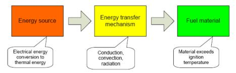
Similar to the use of safeguards in the model for protection against pain/injury, safeguards, such as thermal resistance, as illustrated below, or a fire enclosure to enclose the fire, can be designed into the equipment (system) to reduce the risk of fire. If adequate safeguards are in place, as defined in the Standard in its prescriptive requirements for the safeguards (Clause 6, Electrically-caused fire), the risk of fire will be reduced to acceptable levels.
